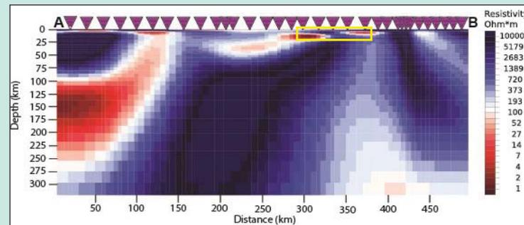
Figure 3: Magnetotelluric subsurface cross section produced from data collected across 33 stations spanning the study region. The highlighted area between the two conductive bodies (yellow box) corresponds to the region of transitioning heat flow shown in Figure 2.
